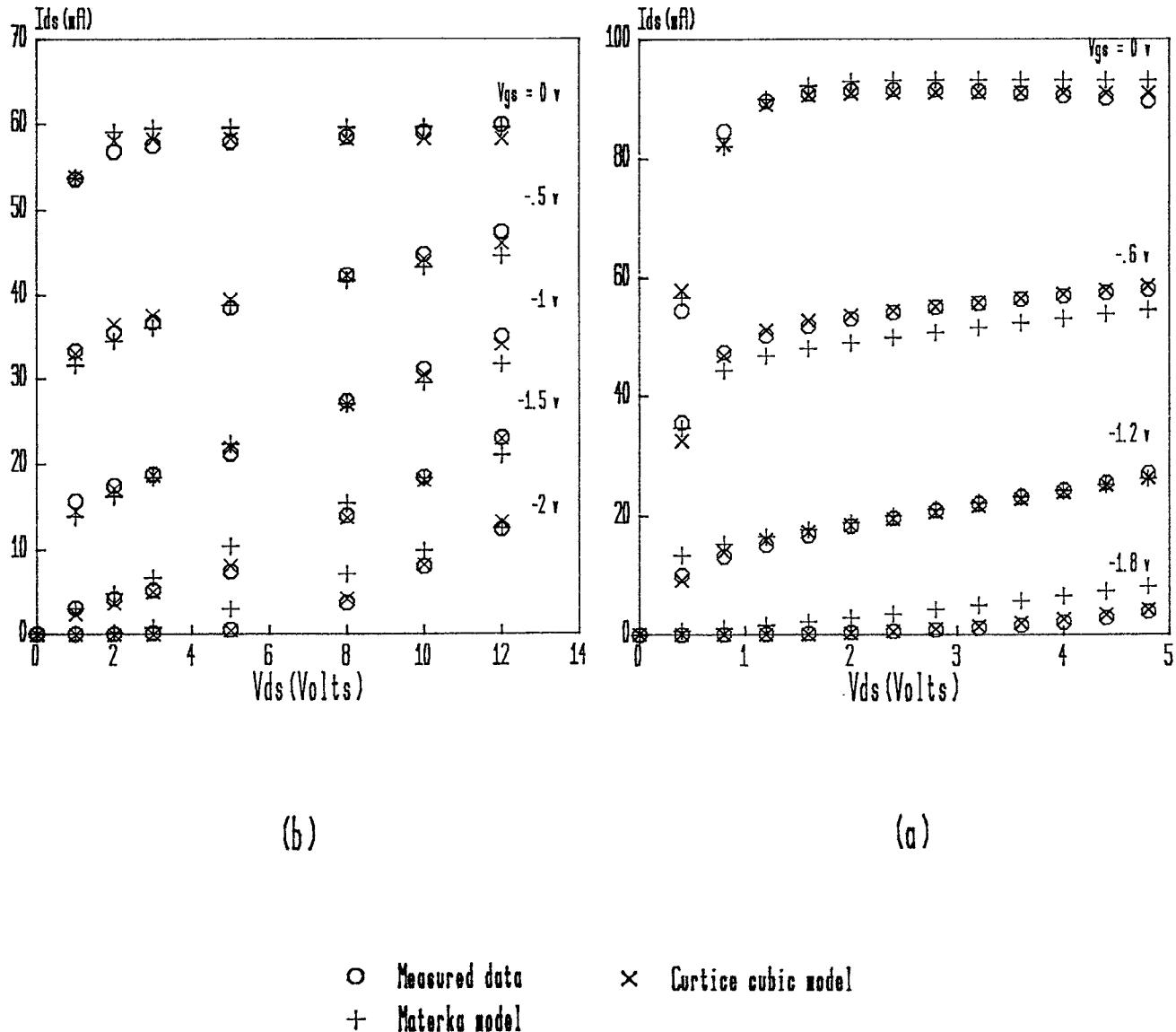
Fig. 1 Comparisons of simulation results and experimental data for MESFETs
